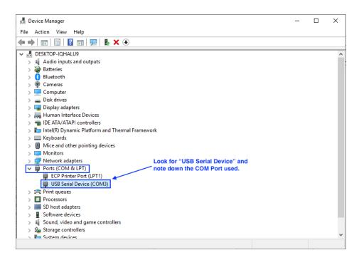
2) Go to "Preferences -> Experiment -> Generic Serial Port". For the "Serial Port One Serial Port" field, select the COM port value identified from the Windows Device Manager. On Mac OS X, the COM Port will appear in the format of "/dev/tty.usbserial-\*\*\*".
