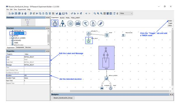
4) At the beginning of the experiment, the EEG recording is started. Select the "Action" tab of the Component Toolbox and add a BIOMETRIC\_TTL node to the graph. Edit the "Label" and "Message" properties of the node to "START EEG RECORDING". Set the "Recipient Biometric Device" to
