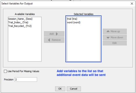
3) Add a NET\_STATION\_CONTROL node from the "Action" tab of the Component Toolbox into the graph and edit the "Label" and "Message" properties of the node. Choose "END TRIAL" from the "Operation" dropdown list. Click the value field of the "Trial Specific (TRSP) Event" property to display a "Select Variables for Output" dialog box, and choose up to 10 project variables to be sent (to avoid flooding the network communication). Then draw a
