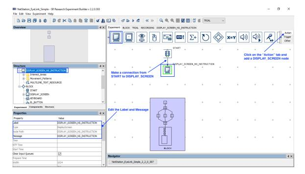
3) Select the newly added DISPLAY\_SCREEN action. Double click to start the Screen Builder. Add a MULTILINE\_TEXT\_RESOURCE to the screen, and enter the desired instruction text.
