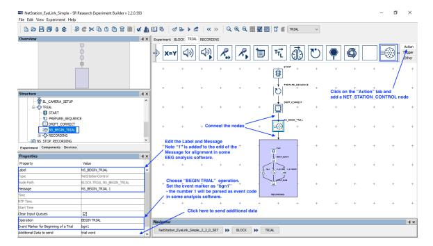
2) The optional property "Additional Data to Send" allows the user to specify any project variables to be sent with the event marker. Click the value field to display a "Select Variables for Output" dialog box, then choose the variables to be sent.
