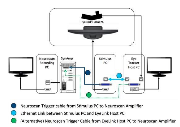
Experiment Builder has built-in functionality to support communication between the Display PC and EEG computer via TTL. The new BIOMETRIC\_TTL action introduced in version 2.2 of Experiment Builder offers more flexibility than the existing SET\_TTL action, and simplifies integration with Neuroscan EEG. This example uses the parallel port of the Display PC to send TTL signals, but the BIOMETRIC\_TTL action also
