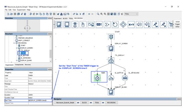
4) Next, send a TTL signal following each of the possible response methods. Let's start with the TIMER trigger. Select the "Action" tab of the Component Toolbox and add a BIOMETRIC\_TTL action. Set the Message of the action to
