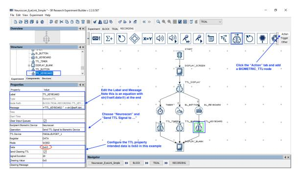
7) Finally, send a TTL signal when the end-of-trial blank screen is displayed. Select the "Action" tab of the Component Toolbox and add a BIOMETRIC\_TTL action. Set the Message of the action to ="TTL\_BLANK" + str(@self.data@), and "Data" to 0x64. Draw a connection from the DISPLAY\_BLANK node to TTL\_BLANK.
