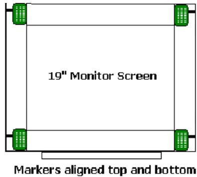
**Figure 2-1: Marker Set-up on EyeLink II Display Monitor**
