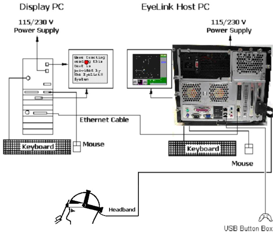
Figure 1-5: System Set-up and Cabling
