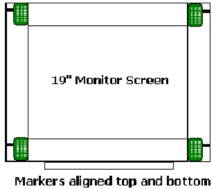
**Figure 1-4: Marker Set-up on EyeLink II Display Monitor**
