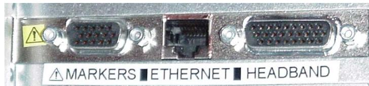
**Figure 1-2 EyeLink II PCI Card Connectors**
